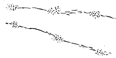
Example of chloride corrosion in stainless steel.
